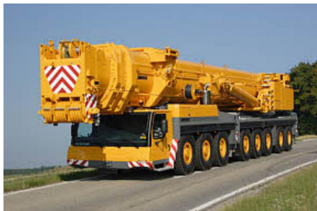
Plate 3.5: Crane for wind turbine erection 2
